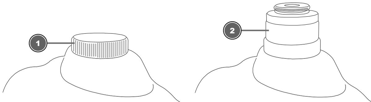
Illustration 3: Trinocular head and attached photo adapter
